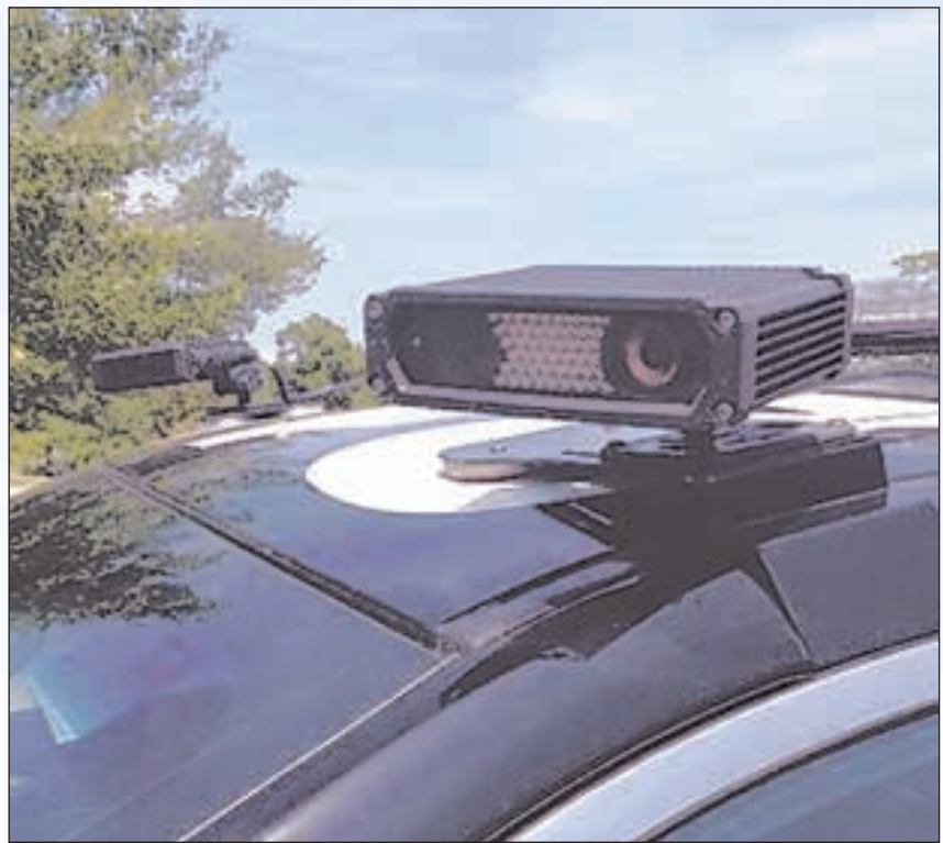
Shown is an example of one type of license plate recognition camera that is mounted to the roof of cruisers. Courtesy Photo
